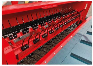
Heavy rotor with 6 rows of pick-up tines
