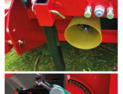
The clutch lever is always pulled up against the welded stop, which ensures full clutch engagement for maximum pulling capacity. This also positions the 3 clutch pins in the correct position for optimal performance.
