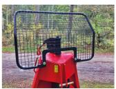
All Fransgård's forest winches are fitted with a safety screen to protect the tractor during work operations . The screen is attached with bolts, which can be easily removed when servicing the machine.
